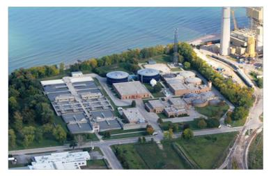
The WWTP is a conventional activated sludge wastewater treatment facility which
